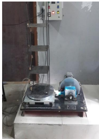
Figure 2: Setup without tuned liquid damper
