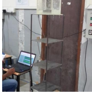
Figure 1: Experimental setup for tuned liquid damper
